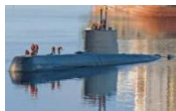
ULA CLASS 4 BOATS (MODIFICATION) THYSENKRUPP MARINE SYSTEMS NORWEGIAN NAVY Delivery: 2007-2008 1.150T – 59m
