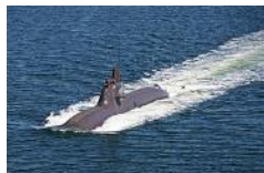
212A CLASS 6 VESSELS THYSENKRUPP MARINE SYSTEMS GERMAN NAVY Delivery: 2002-2011 1.830T – 57m
